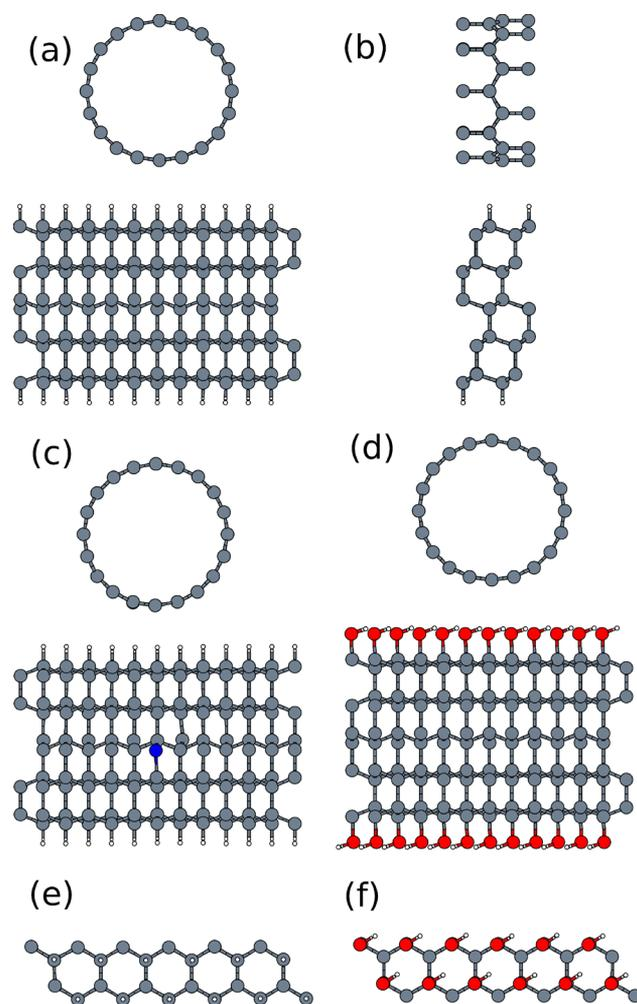
**Figure 1.** Geometry of the used supercells. Panels a and b show the front and side views of a (10,0) SCNT on hydrogen-terminated diamond, respectively. Panel c shows an N-doped system in which a carbon atom was replaced by nitrogen. Panel d shows the (10,0) SCNT atop OH-terminated diamond. Panels e and f show the optimized surface layer of H-terminated diamond and OH-terminated diamond, respectively.
