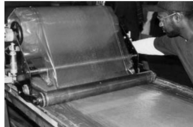
Figure Prepreg Ply of E-Glass is Rolled Out on Consolidation Table by Composite Ships
