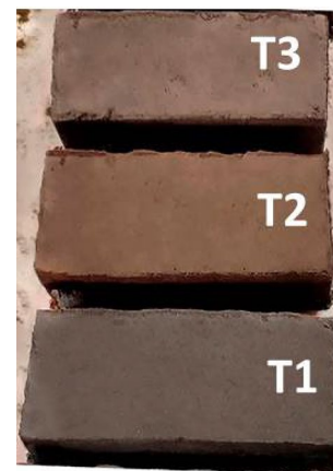
Fig. 1 Bricks made from waste steel (T365) and iron mining (IOT) and cement. T1, T2 and T3 are the respective proportions of raw materials: T1 (100/0/0), T2 (85/15/0) and T3 (85/10/5)
