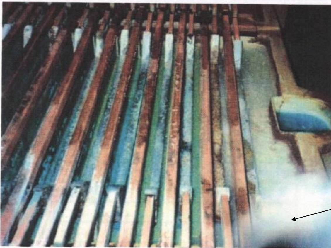
Surface of a typical copper electrowinning cell showing polymer beads.
